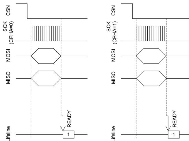
**Figure 152: SPI master transaction**
