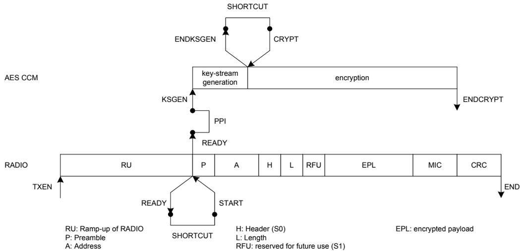
**Figure 63: On-the-fly encryption using a PPI connection**
