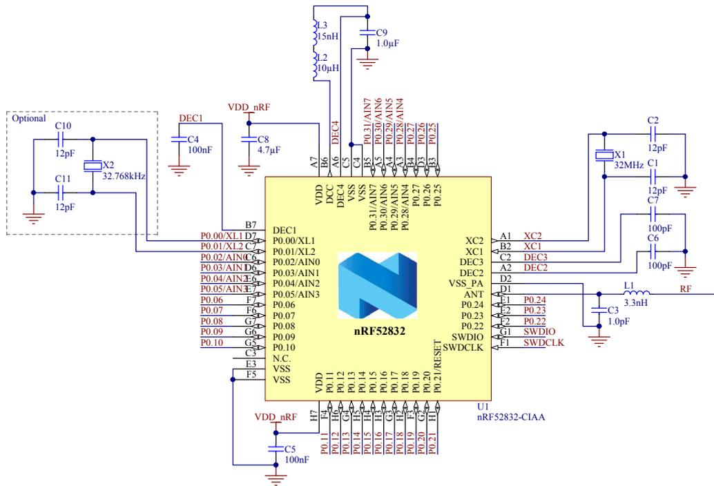
Figure 173: CIAA WLCSP with DC/DC regulator setup
