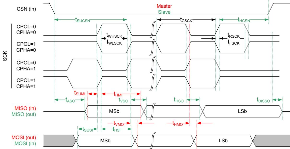
Figure 76: Common SPIM and SPIS timing diagram
