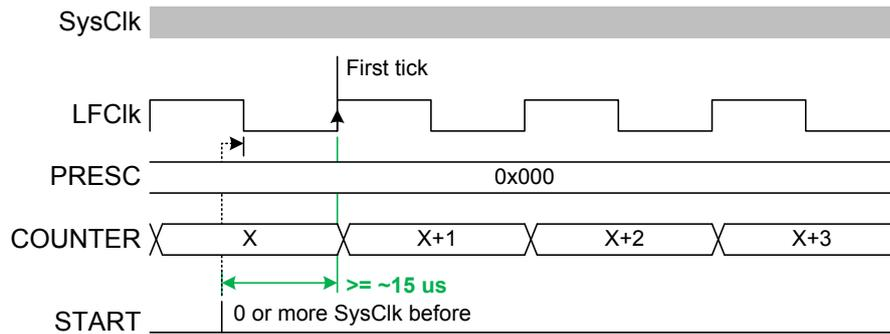
**Figure 55: Timing diagram - JITTER\_START-**
