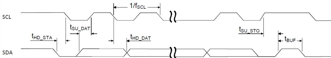
**Figure 159: TWI timing diagram, 1 byte transaction**
