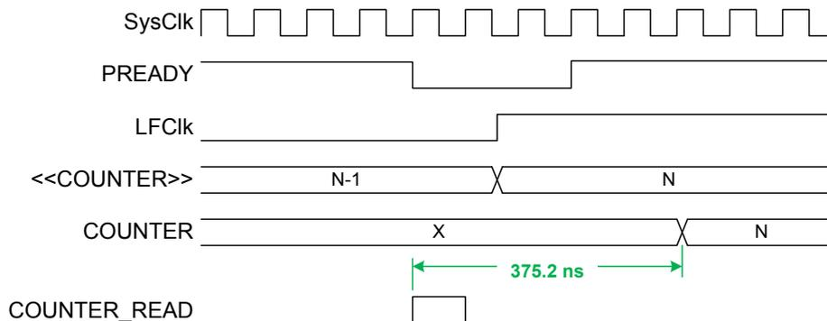
**Figure 57: Timing diagram - COUNTER\_READ**
