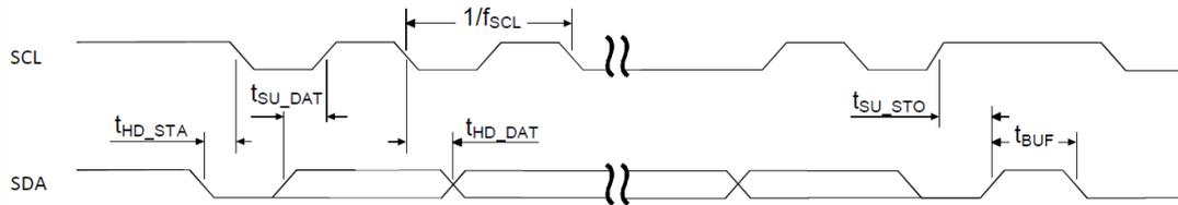
Figure 92: TWIS timing diagram, 1 byte transaction
