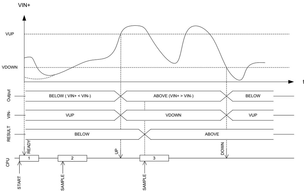
Figure 113: Hysteresis example where VIN+ starts below VUP
