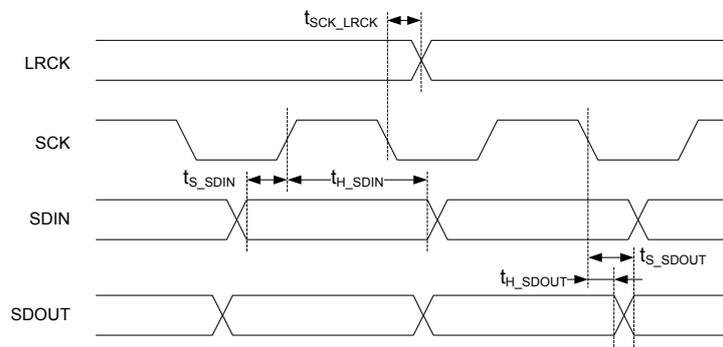
Figure 140: I2S timing diagram
