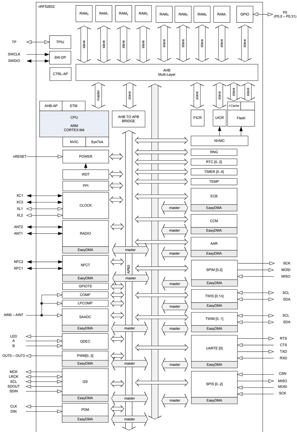
Figure 1: Block diagram
