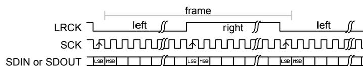
**Figure 132: I<sup>2</sup>S format. CONFIG.SWIDTH equalling half-frame size.**
