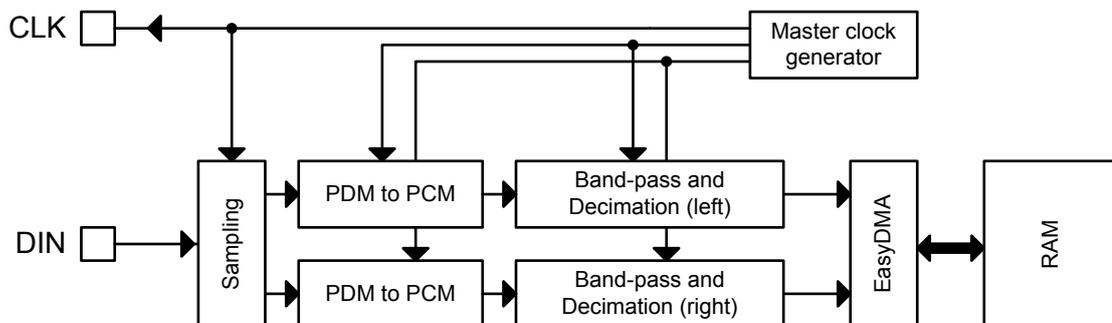
Figure 124: PDM module
