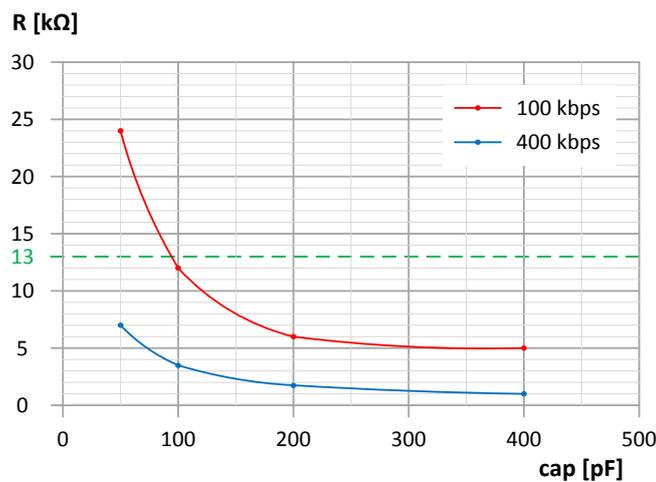
Figure 85: Recommended TWIM pullup value vs. line capacitance
