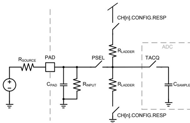
**Figure 105: Model of SAADC input (one channel)**
