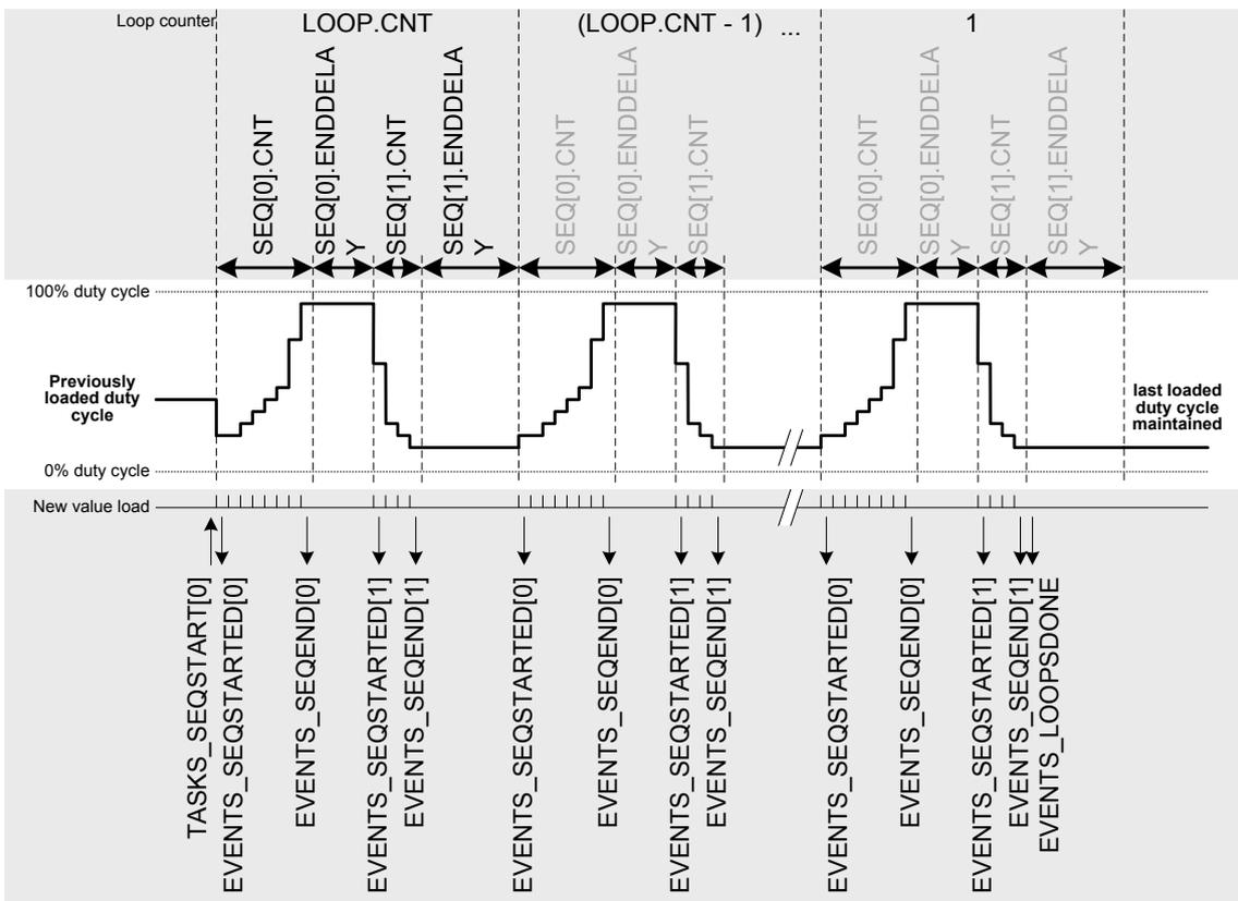
Figure 148: Complex sequence (LOOP.CNT>0) starting with SEQ[0]
