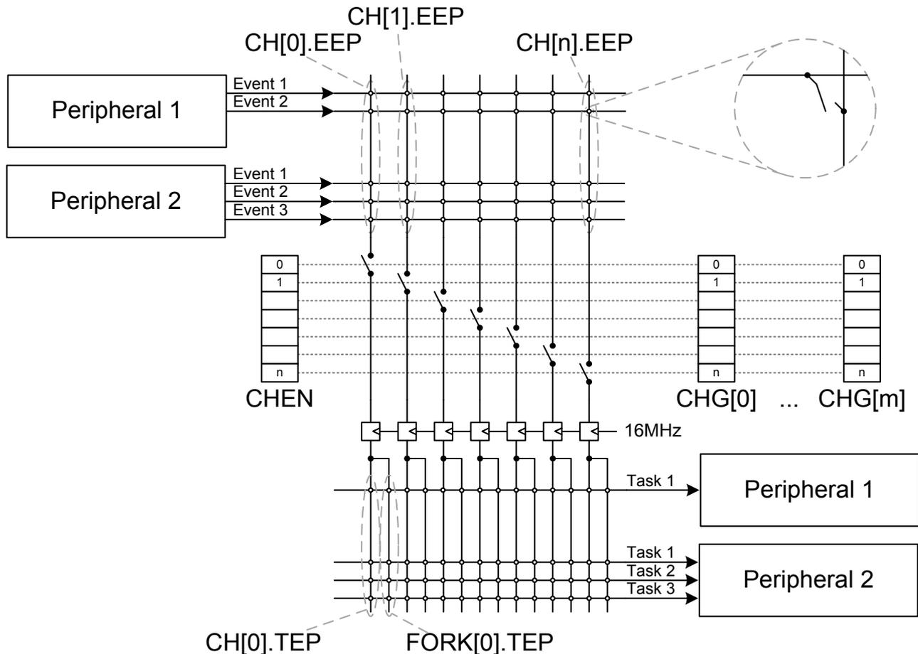
**Figure 28: PPI block diagram**
