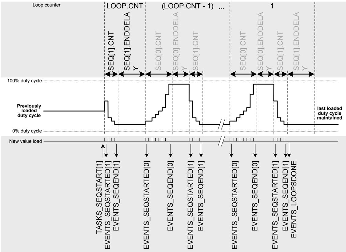
**Figure 149: Complex sequence (LOOP.CNT > 0) starting with SEQ[1]**
