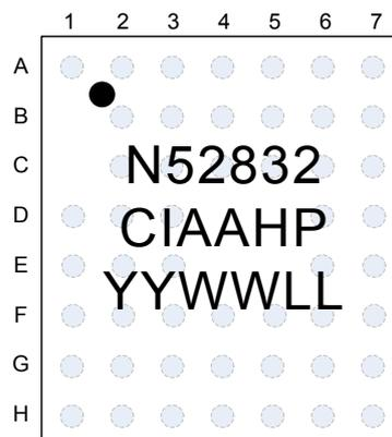
Figure 3: WLCSP ball assignments, top view
