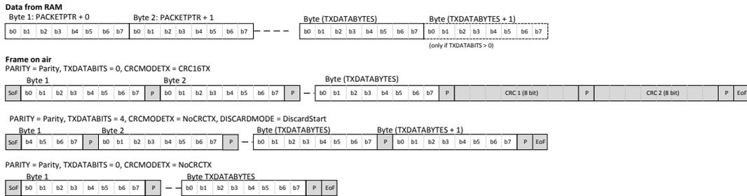
**Figure 120: Frame assemble**
