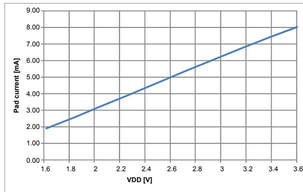
Figure 25: Max sink current vs Voltage, standard drive
