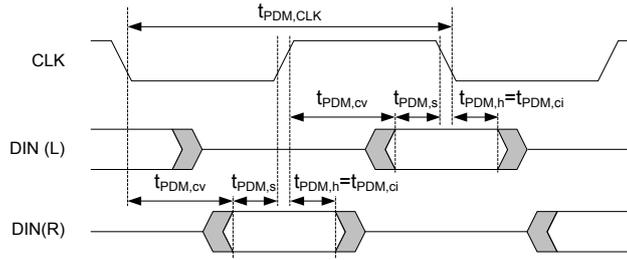
**Figure 128: PDM timing diagram**
