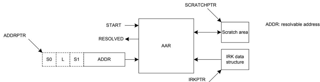
Figure 67: Address resolution with packet preloaded into RAM
