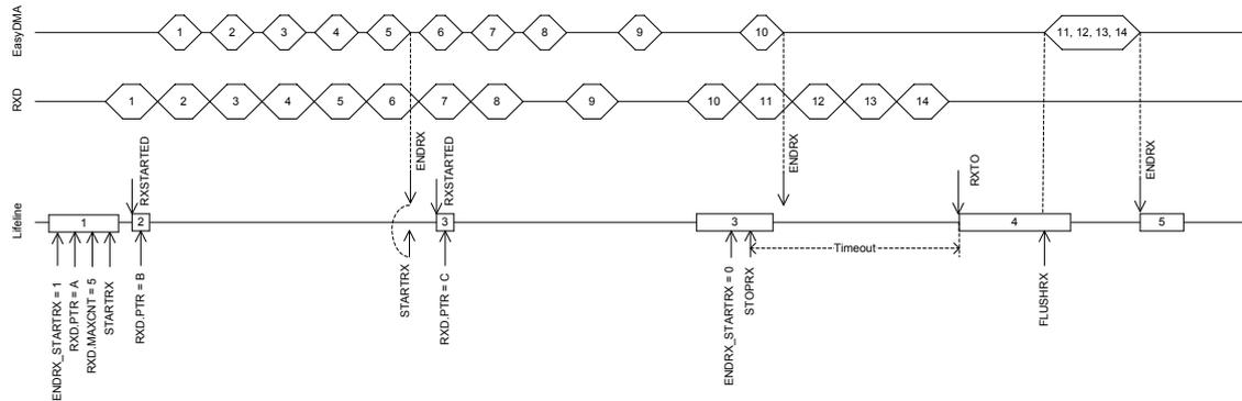
**Figure 96: UARTE reception with forced stop via STOPRX**
