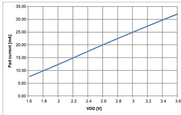
Figure 26: Max sink current vs Voltage, high drive
