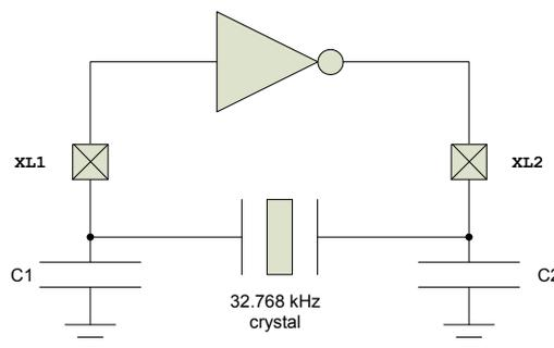
**Figure 20: Circuit diagram of the 32.768 kHz crystal oscillator**
