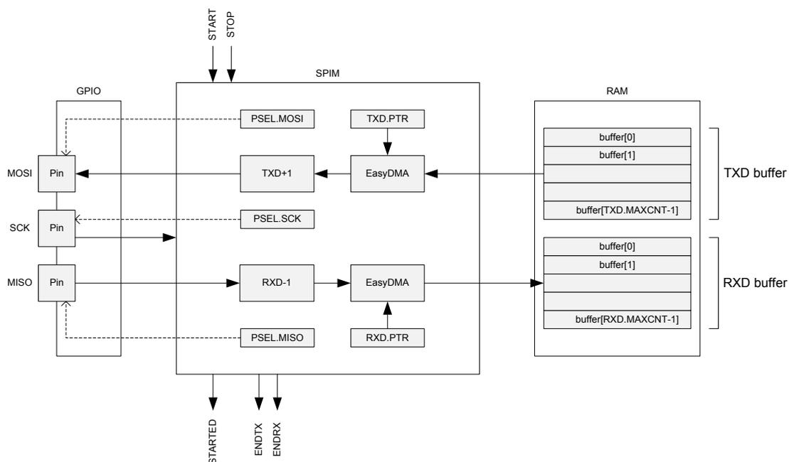
**Figure 69: SPIM — SPI master with EasyDMA**
