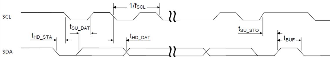
Figure 84: TWIM timing diagram, 1 byte transaction
