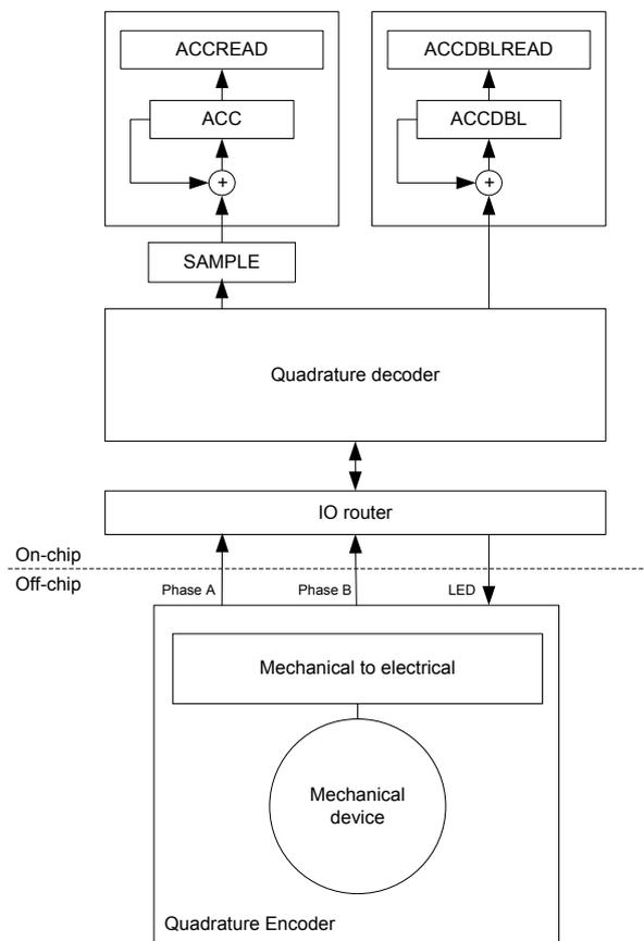
Figure 97: Quadrature decoder configuration
