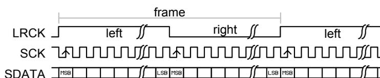
**Figure 133: Aligned format. CONFIG.SWIDTH equalling half-frame size.**
